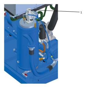
Fig. 11: Minimum pressure and non-return valve
