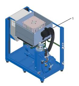
Fig. 40: intake filter
