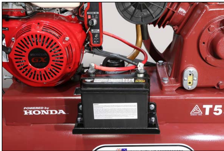
Figure 5-8 Airmac 12 Volt Battery Kit Installed
