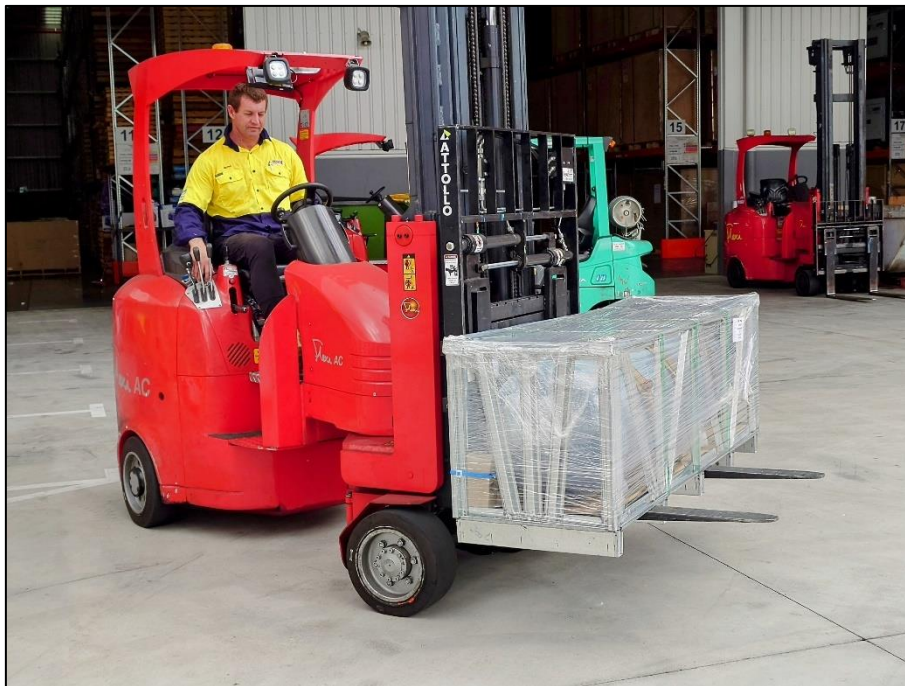
Figure 4-1 Forklift Handling of a Packed Vertical Air Receiver
