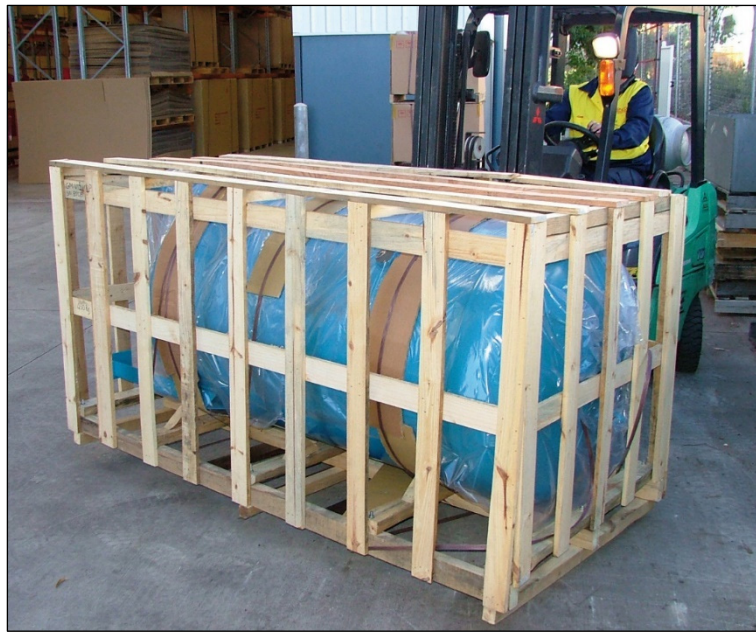
Figure 4-1 Forklift Handling of a Packed Vertical Air Receiver
