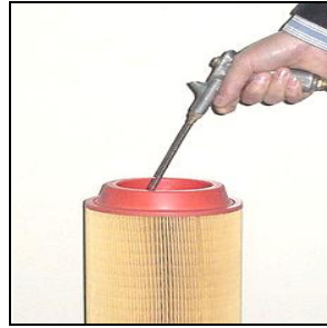
Figure 8 Air Filter Element Cleaning
