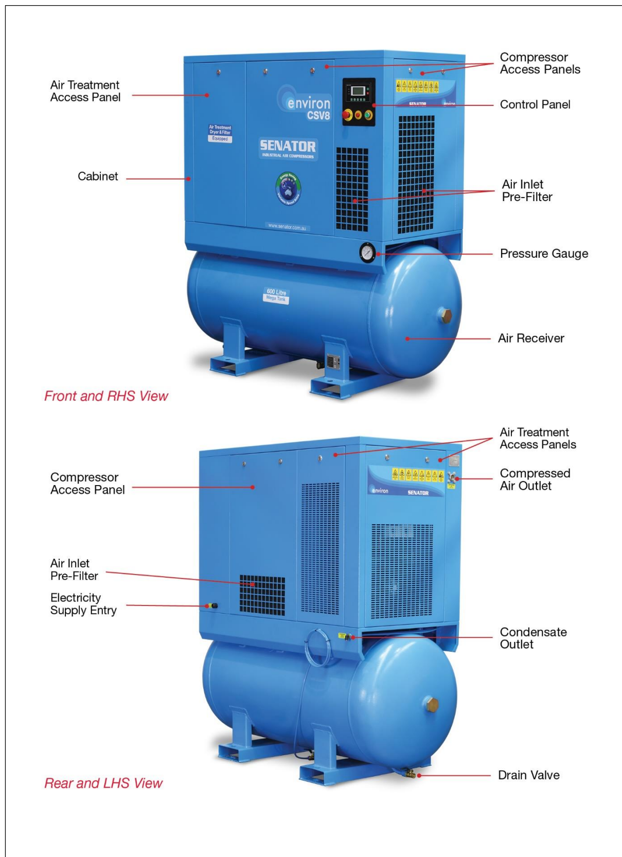
Figure 3-2 External Features of CSV Series Air Compressor Set
