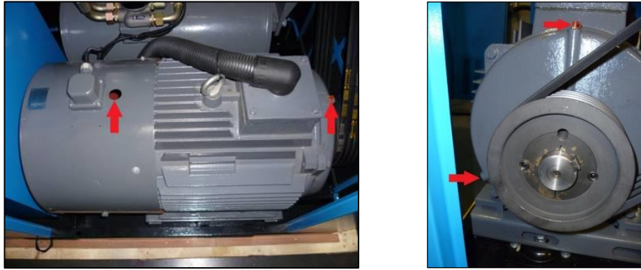
Figure 6-7 Motor Bearing Re-Greasing
