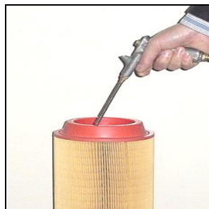
Figure 6-3 Air Filter Element Cleaning
