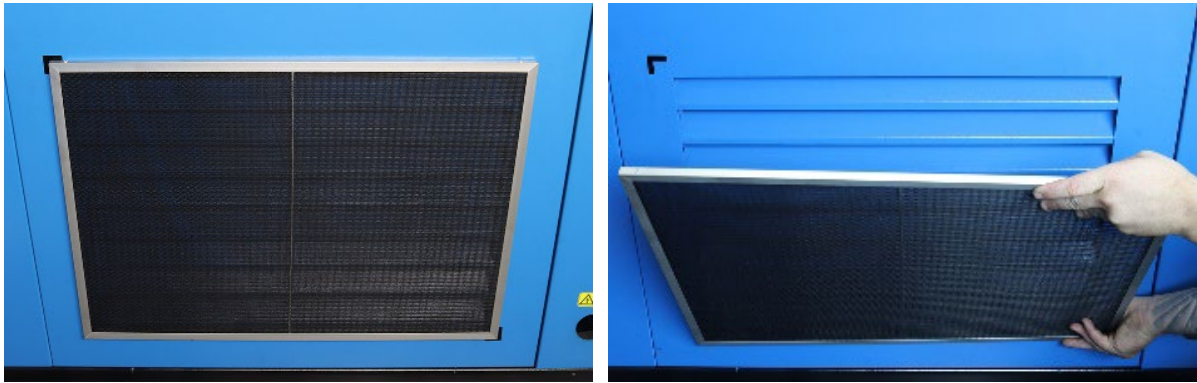
Figure 7 Air Pre-Filters Location and Removal
