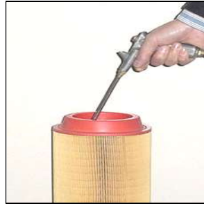
Figure 6-3 Air Filter Element Cleaning
