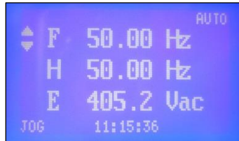
Figure B-3 VSD Display in AUTO Mode
