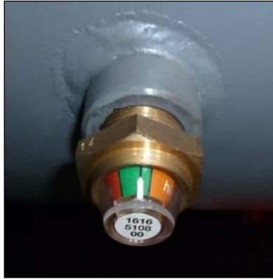
Figure 6-1 Full Oil Level Indication
