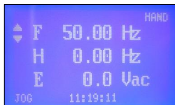
Figure B-4 VSD Display in HAND Mode
