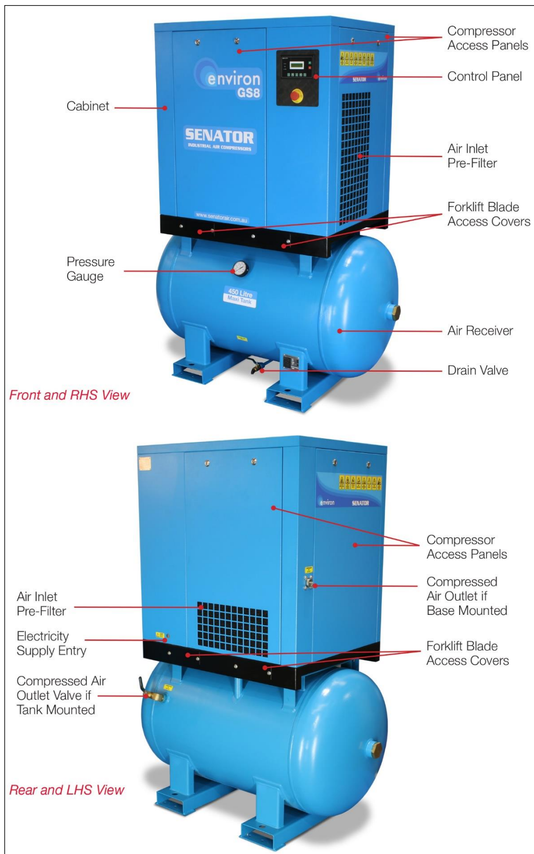
Figure 3-2 External Features of GS Series Air Compressor Set
