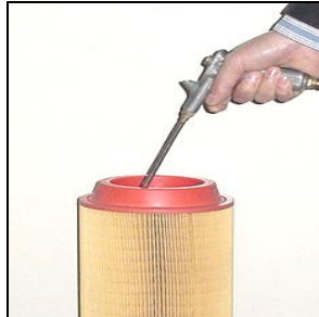
Figure 6-3 Air Filter Element Cleaning
