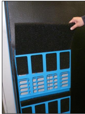
Figure 6-2 Air Pre-Filters Removal
