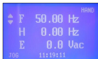
Figure B-4 VSD Display in HAND Mode
