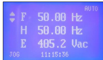
Figure B-3 VSD Display in AUTO Mode
