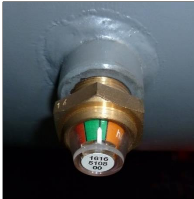
Figure 6-1 Full Oil Level Indication
