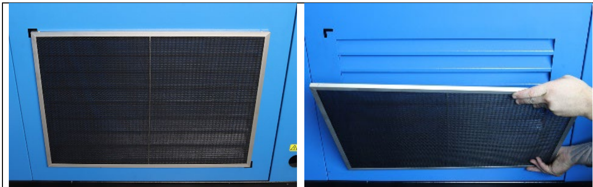
Figure 7 Air Pre-Filters Location and Removal
