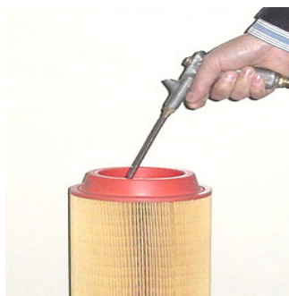
Fig. 4.2 Air Filter Element Cleaning
